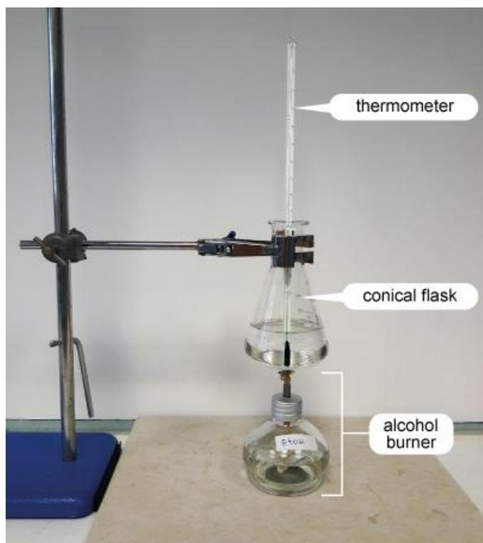
**Figure 4.** Simple calorimeter used to determine heat energy released in the combustion of alcohols.
