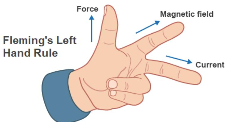
**Figure 1** The use of Fleming's Left Hand Rule.
