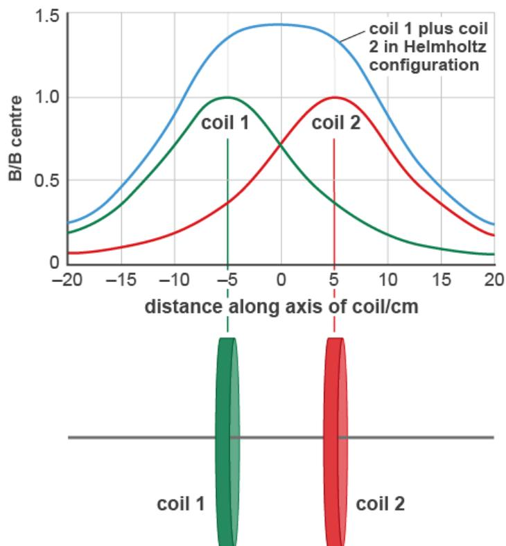
**Figure 2** A graph showing the magnetic field strength along the axis of two identical coils aligned coaxially, and separated by a distance equal to their radius of 10 cm. The lower curves represent the field strength due to each coil individually, which each has a peak at
