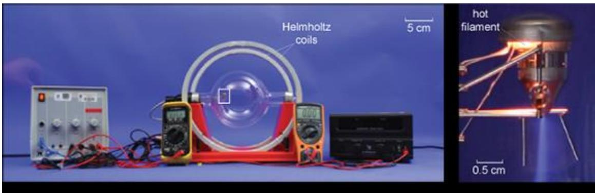
**Figure 5** From left to right you can see the power supply used to accelerate the electrons, voltmeter (measures voltage), fine beam tube within the two coils, ammeter (measures current) and power supply to the coils. On the far right you can see a close-up of the lilac beam emerging downwards from the hot cathode (its location within the glass tube is indicated by the white rectangle).
